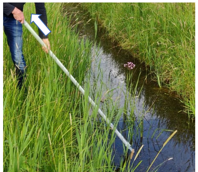
Figure 3. Taking water samples using the eDNA dual filter capsule without ( A ) and with ( B ) sampling rod.
