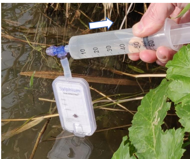
Figure 3. Taking water samples using the eDNA dual filter capsule without ( A ) and with ( B ) sampling rod.
