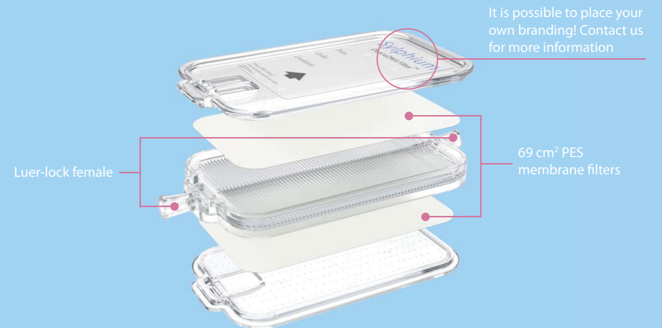
Exploded view of the eDNA Dual Filter Capsule
